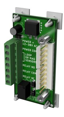
Many vehicle detectors are designed to be plugged into a rack including some of the more popular Diablo Controls models. In those installations where a large rack is not available, Diablo Controls has designed a mini rack. The RK-1R is designed to accept a plug-in vehicle detector on one side and accept the appropriate wires through the terminal block on the other. The entire mini rack is supported by four adhesive standoffs that attach anywhere in the cabinet.
