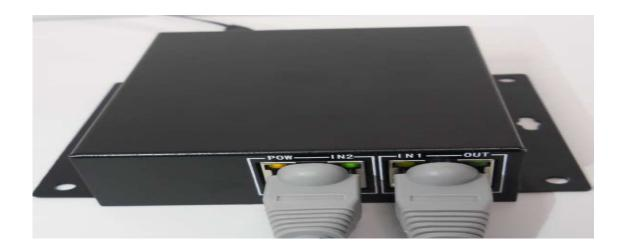
6. Using the supplied DC cable, connect the ZKAccess PoE Splitter to the ZKAccess panel's power/pigtail. This completes the installation.
