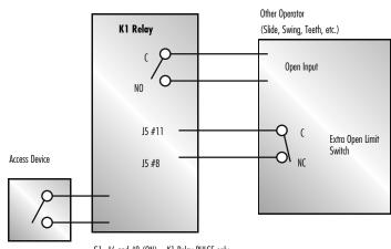
S1, #6 and #8 (ON) = K1 Relay PULSE only. S1, #6 and #8 (OFF) = K1 Relay LATCH only.
