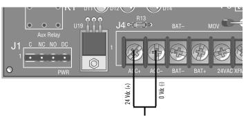
Relay Connection Terminals on the J4 Terminal Block
