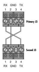
**IRD** - Obstruction Signal Connections Terminal 1 of Primary must go to terminal 4 of Second and terminal 1 of Second must go to terminal 4 of Primary. Terminal 2 of Primary must go to terminal 2 of Second.
