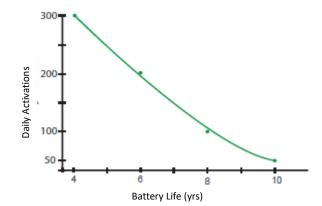
Note: Battery life is dependent on many factors, including daily activations, time used per activation, radar range and external conditions.
