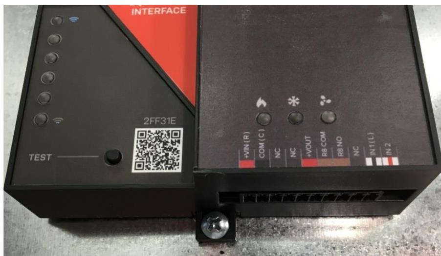
Figure 23: Equipment Interface with the relay COM of R6, R7, and R8 shown wired to +VOUT
