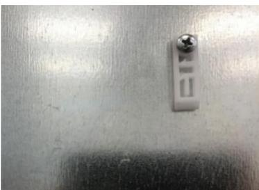
Figure 21: The DIN clip on the top is shown secured with a #8 screw and the base reconnected to the DIN clip.
