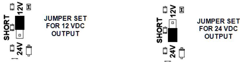
Power Module Output Power Jumper Settings (only on models with lock power)
