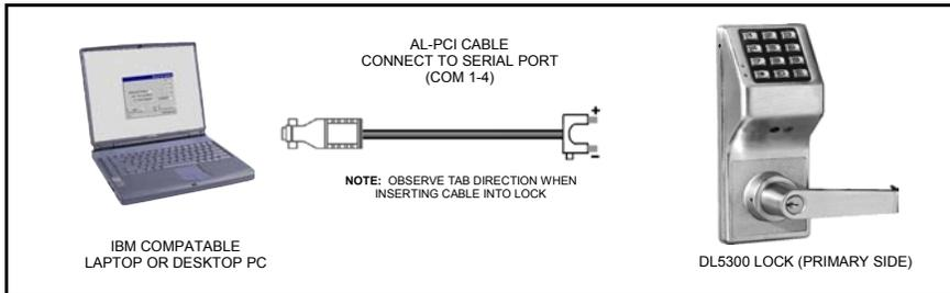
If your computer does not have a serial COM port (DB-9 male) available, you can plug your AL-PCI2 cable into a special USB to RS-232 cable. Order part **MX1130** for the USB to RS-232 cable only, or **ALPCI2-U** for both the USB to RS-232 cable and an AL-PCI2 cable.
