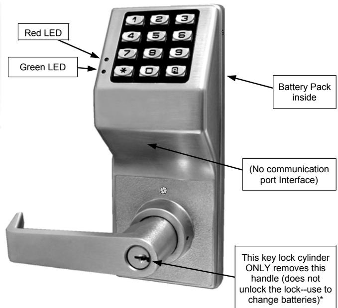
\* **Note:** Only the Primary Lock Side key cylinder allows non-logged access; the Secondary Lock Side cylinder is only used to secure the housing to the door. Therefore a person in possession of only the metal key on the Secondary Lock Side has no means of unlocking the DL5300 lock.
